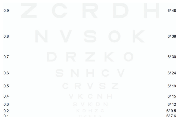
FIGURE 8 Contrast sensitivity function showing the approximate relationship between high and low contrast visual acuity and letter contrast sensitivity (image courtesy of Thomson Software Solutions)
